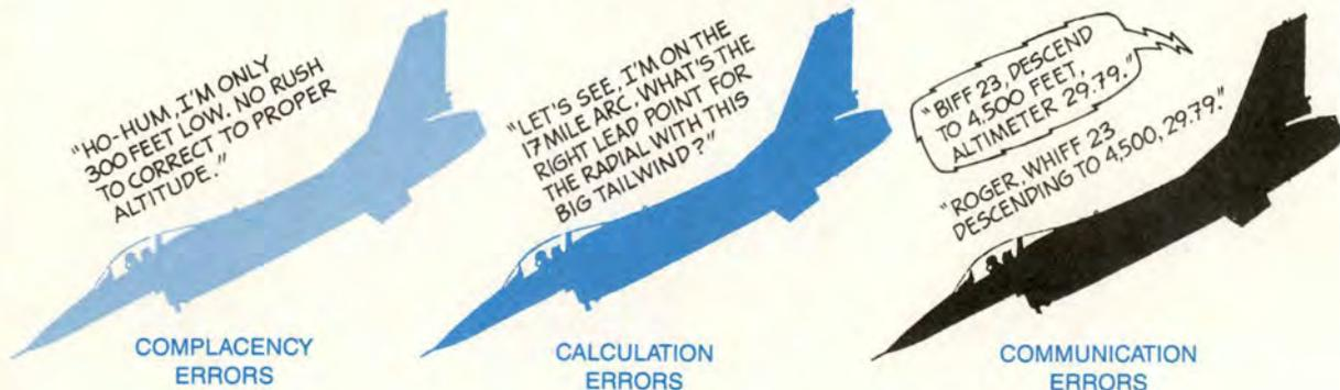
When a pilot is fatigued, his performance will be degraded in a predictable pattern consisting of the following triad: Increased complacency, calculation errors, and communication misinterpretations.
